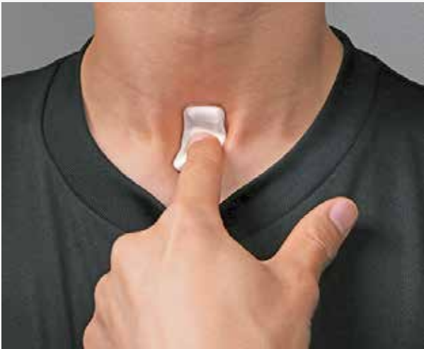
→ A wearable sensor sits at the throat to monitor coughs, fever and respiratory activity.
